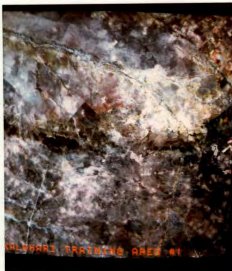
Plate 1 Photograph of portion of false colour composite Landsat image WRS 185-79 (bands 4, 5 and 7; summer) representing the Kalahari Thornveld Training Area. Originally at a scale of 1: 250 000.
