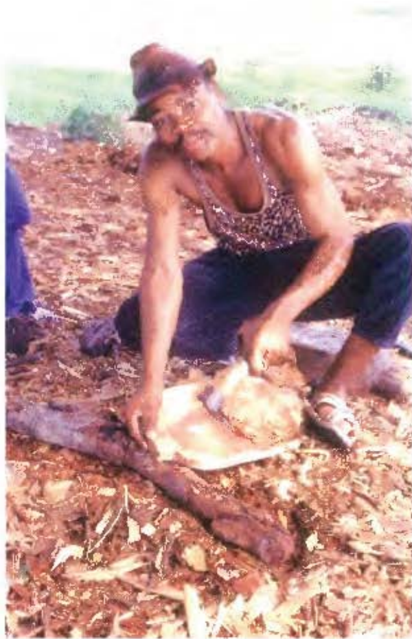
Plate 22 Crafters chop the bowls into shape using a rough hoe-like tool. The pile of wood chippings beneath this crafter has been generated over many months of bowl construction.
