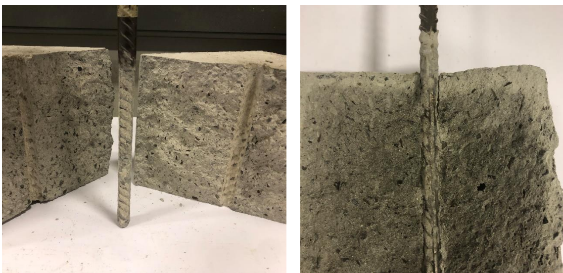
Figure 42: Splitting failure with coating shear for 10% corroded specimens
