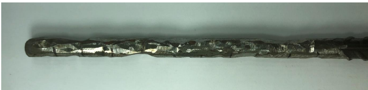
Figure 21: 20% cleaned corroded steel
