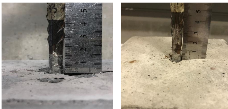
Figure 37: (a) Untreated 20% corroded steel with 15 mm slip, and (b) 30 – 35 mm slip
