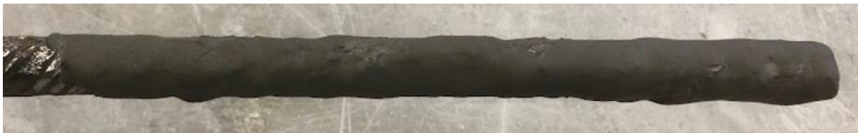
Figure 41: 10% corroded steel with two coats
