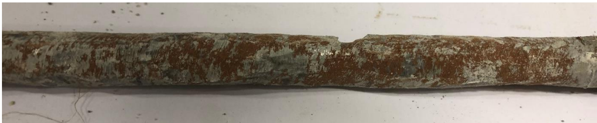
Figure 38: Corrosion effects of untreated steel after 7 days wet curing
