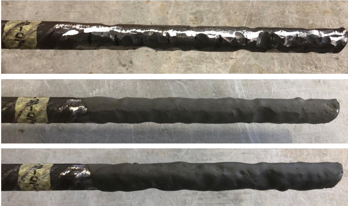
Figure 44: 20% corroded untreated (top), one coat (centre), two coats (bottom)
