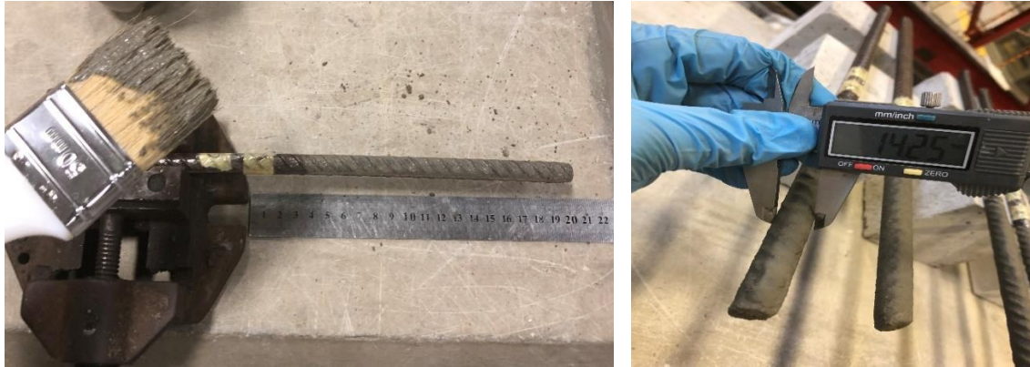
Figure 22: Coating application and thickness measurement
