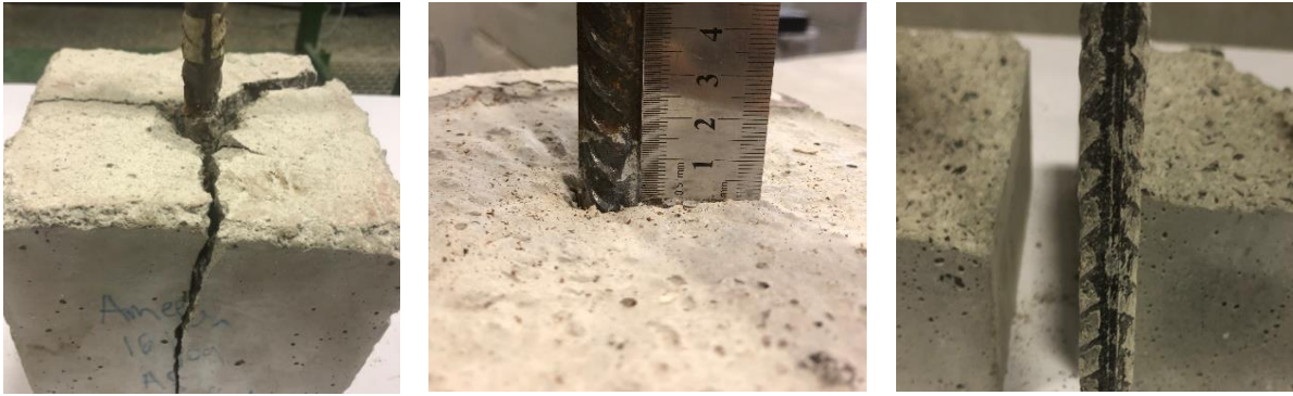
Figure 27: Splitting (a), 15 mm slip (b), splitting with coating failure (c)
