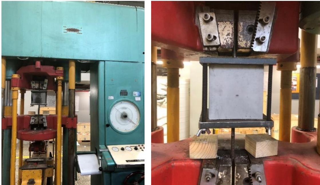
Figure 25: (a) Pull-out test machine (left), and (b) Specimen arrangement (right)
