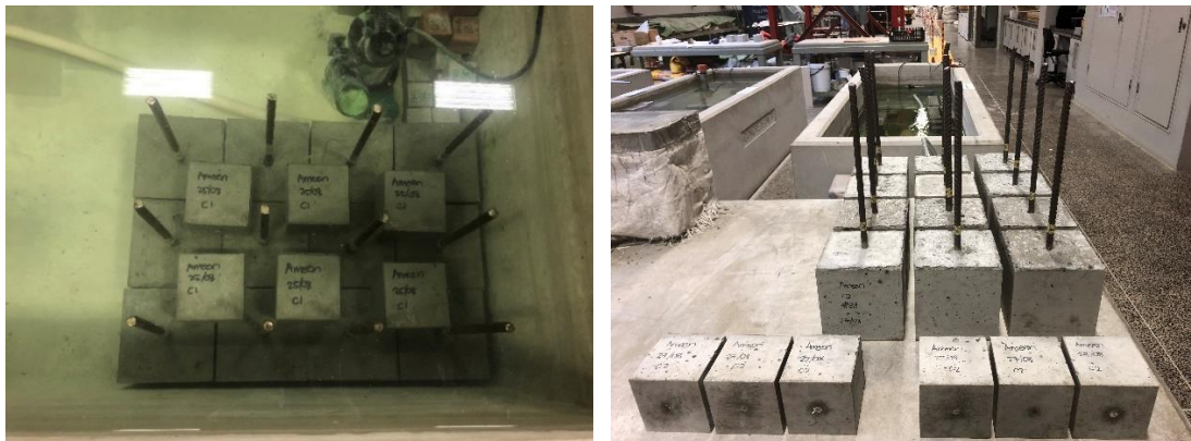
Figure 24: Test specimens after demoulding and curing
