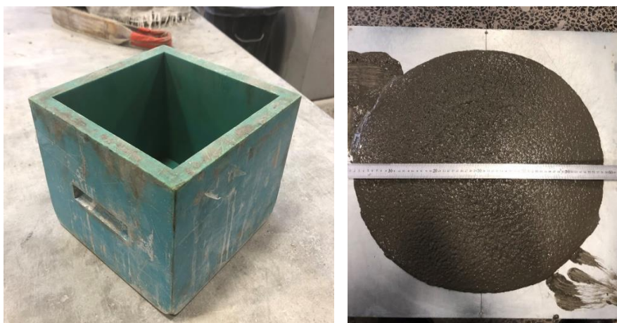
Figure 23: (a) Plastic mould, and (b) mortar flow
