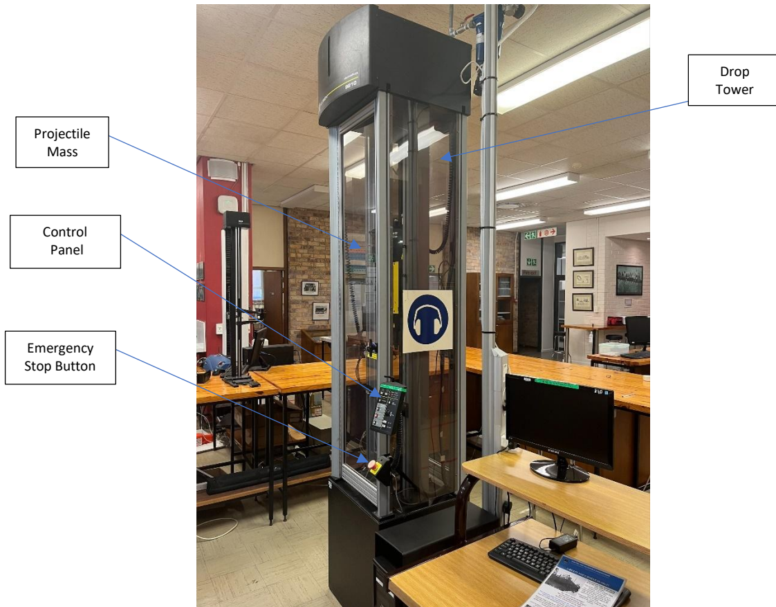
Figure 48: Image of Instron Dynatup 9210 Impact Tester
