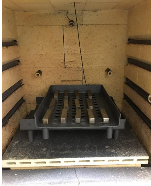
Figure 42: Image of marked pre-heat treated CVN specimens in hot furnace tray
