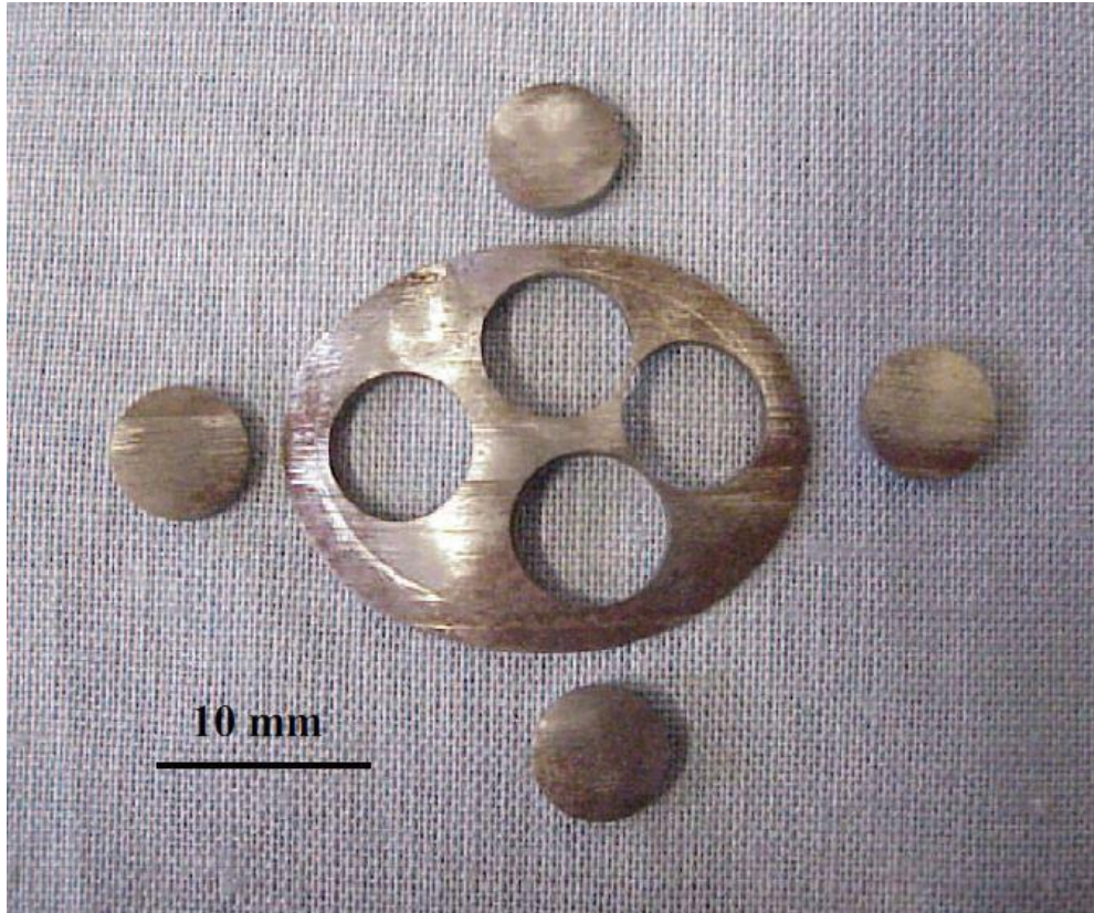
Figure 12: Sample removed by scoop cutter with SPT specimens cut using EDM [24]
