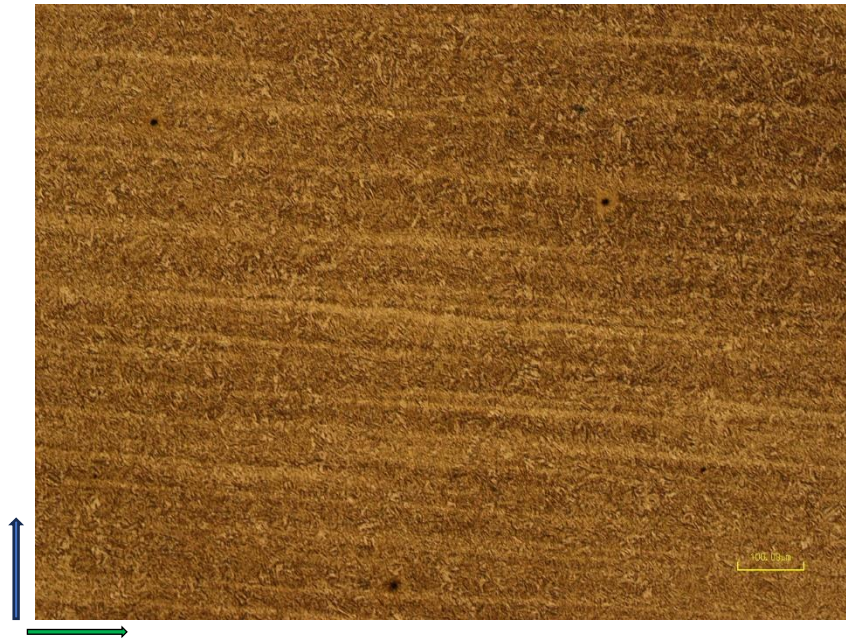
Figure 59: Microscopic image as viewed in the transverse direction of the material displaying the S-L plane (orientation C)
