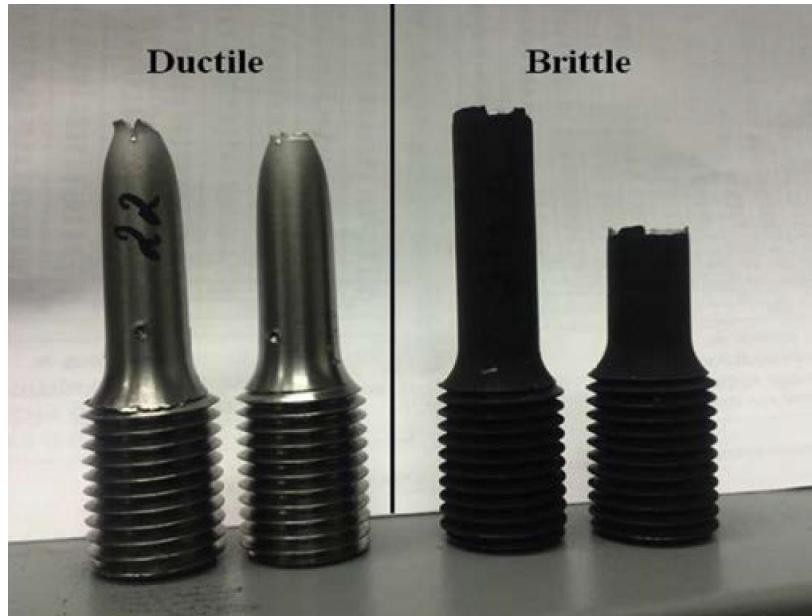
Figure 7: Ductile and brittle failure of steel specimens [23]
