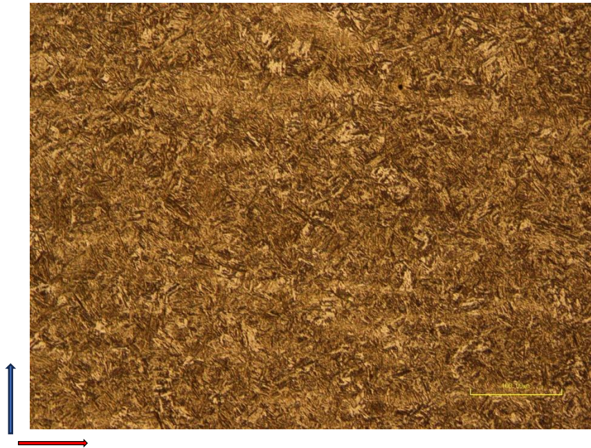
Figure 60: Microscopic image as viewed in the rolling (longitudinal) direction displaying the S-T plane (orientation B)
