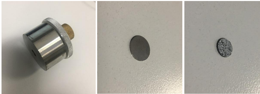
Figure 54: Image of grinding jig, SPT specimen ground to thickness \approx 0.5 mm and speckled SPT specimen ready for testing
