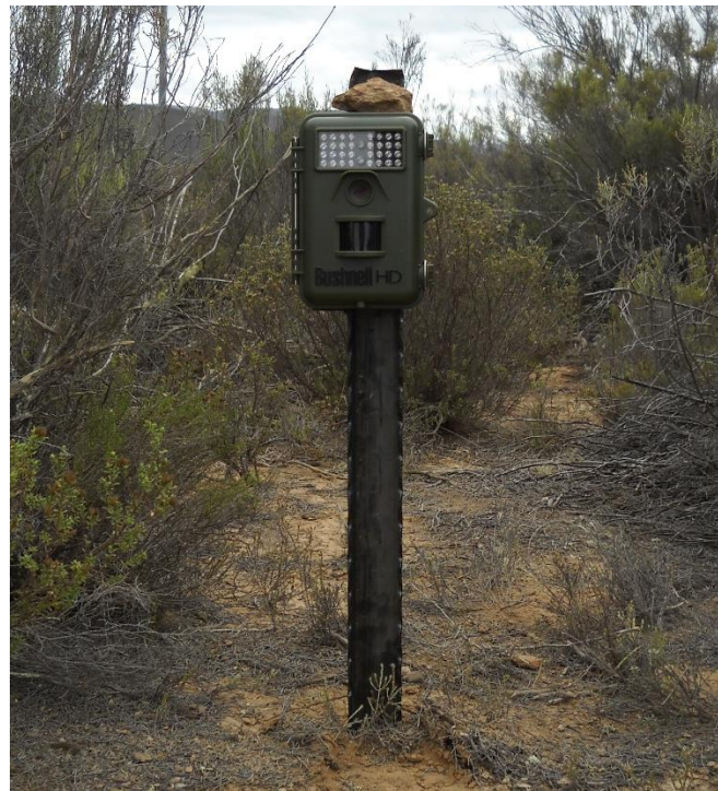
Figure 3.5: Bushnell Trophy CAM HD camera trap mounted on a metal pole.
