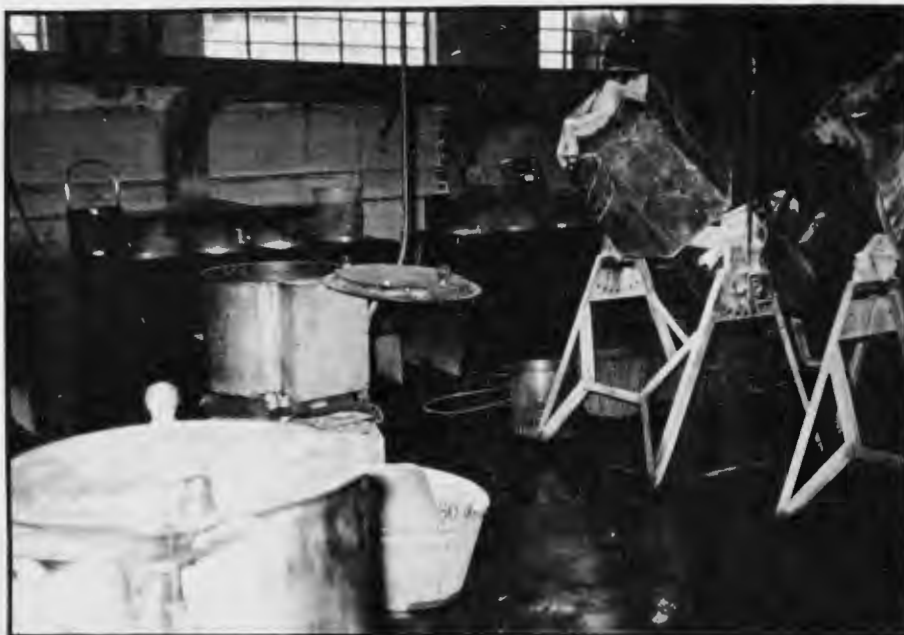
Photograph 1: General view of Processing Area. (Hexagonal Polishing Tumbler on right; Dye Vats against rear wall).
