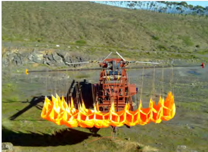
Figure 4.27: Completed Set Up of the Parafoil Launcher
