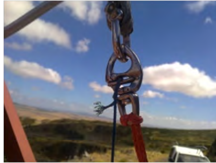
Figure 4.18: Catapult Arm Quick-release Shackle
