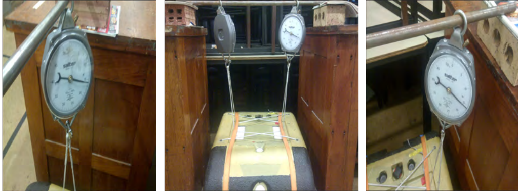
Figure 4.10: Checking Payload Box's Centre of Gravity
