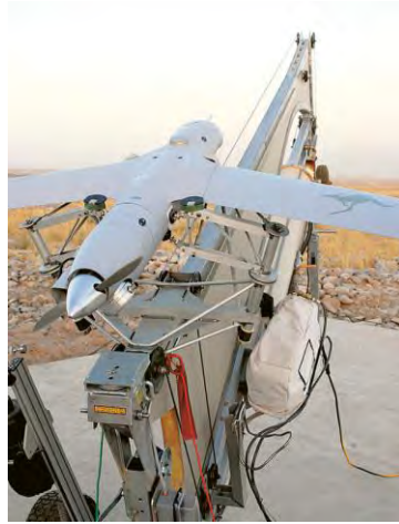
Figure 2.16: Bungee Cord Launching Device [53]
