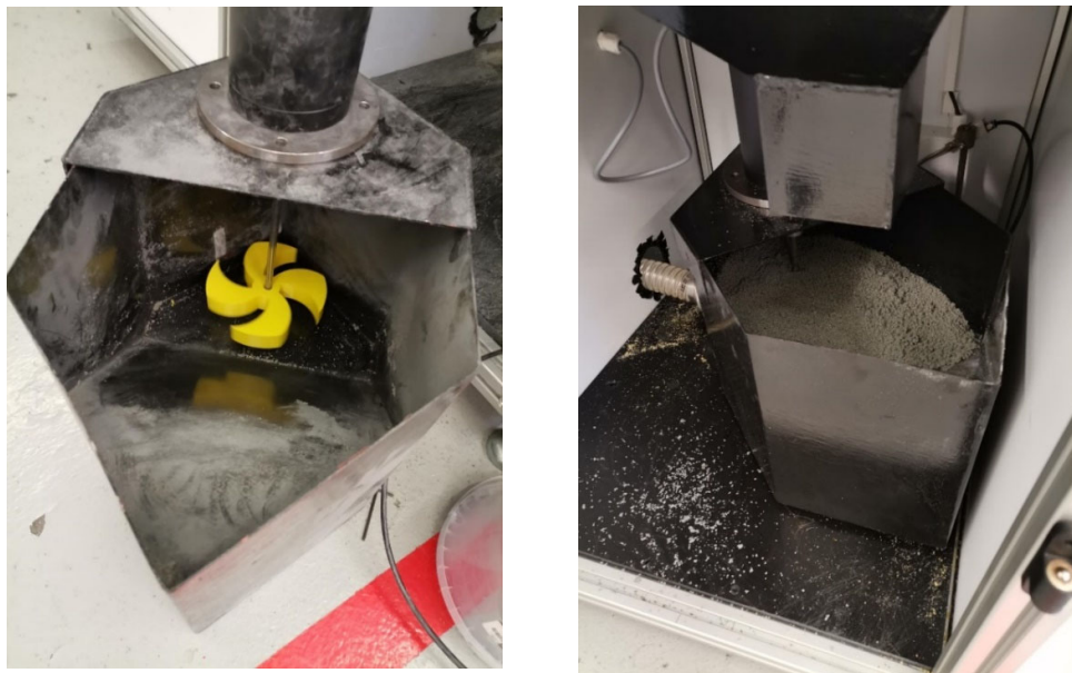
Figure 31 - (a) Empty bin with attached stirrer and stirrer motor (b) Installed subassembly and visible end of hopper as well as a bin full of abrasive media
