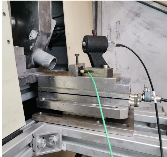
Figure 56 - Dynamometer, Accelerometer and AE Sensor Set-Up
