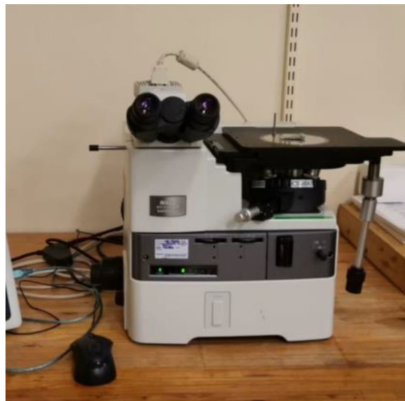
Figure 59 - Nikon Inverted Metallurgical Microscope
