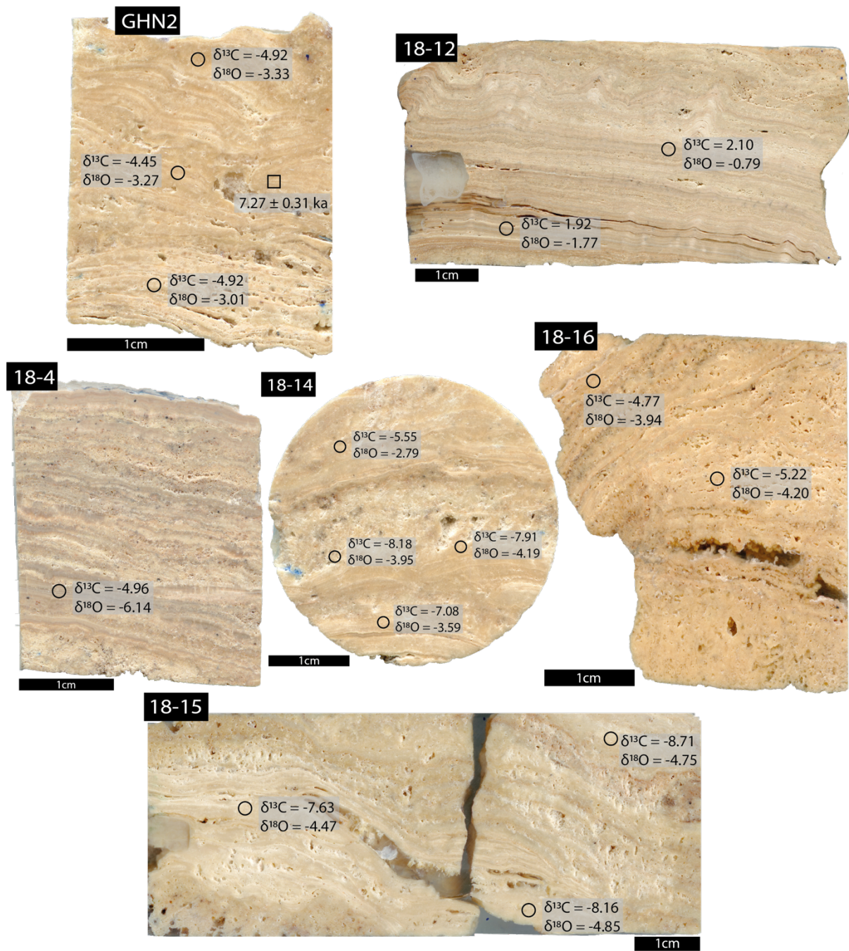
Figure 7.2.4 The \delta^{18}\text{O}_{\text{PDB}} and \delta^{13}\text{C}_{\text{PDB}} values of material drilled at the indicated position for cascade samples GHN2, 18-12, 18-4, 18-14, 18-16 and 18-15.
