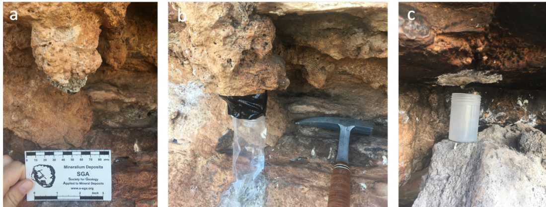
Figure 3.1.3 Photographs from water collection at Ga-Mohana Hill: a) actively dripping micro-stalactite, b) plastic bag strapped to dripping micro-stalactite, c) plastic bottle positioned on a ledge beneath a drip.
