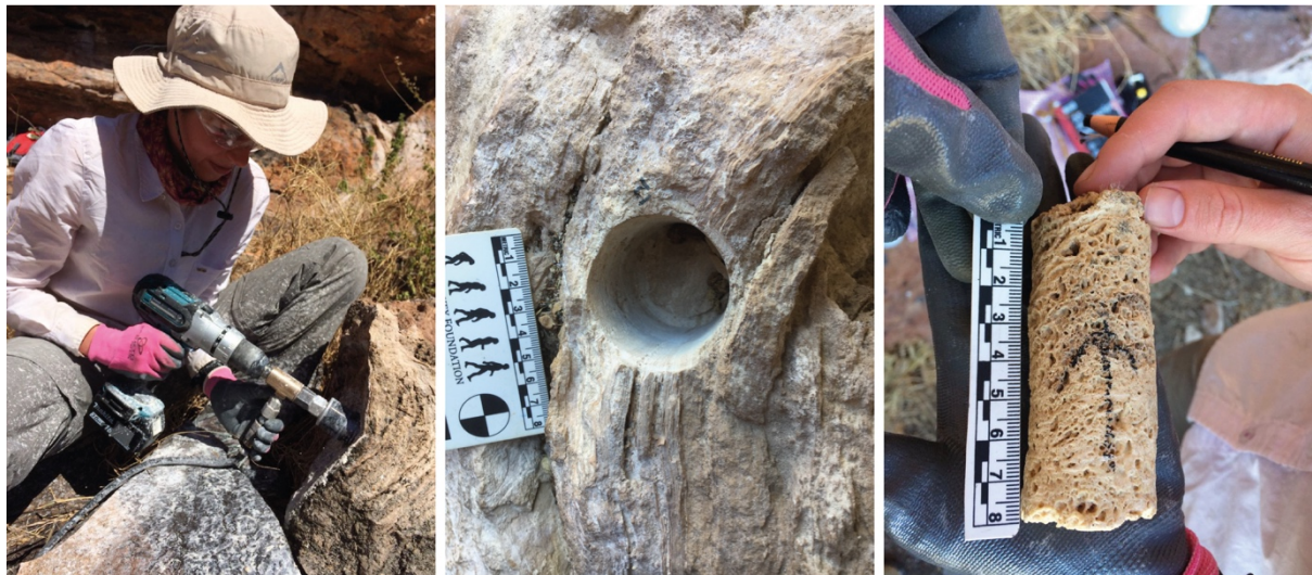
Figure 3.1.2 Sampling of tufa using modified hand drill fitted with custom core barrel.
