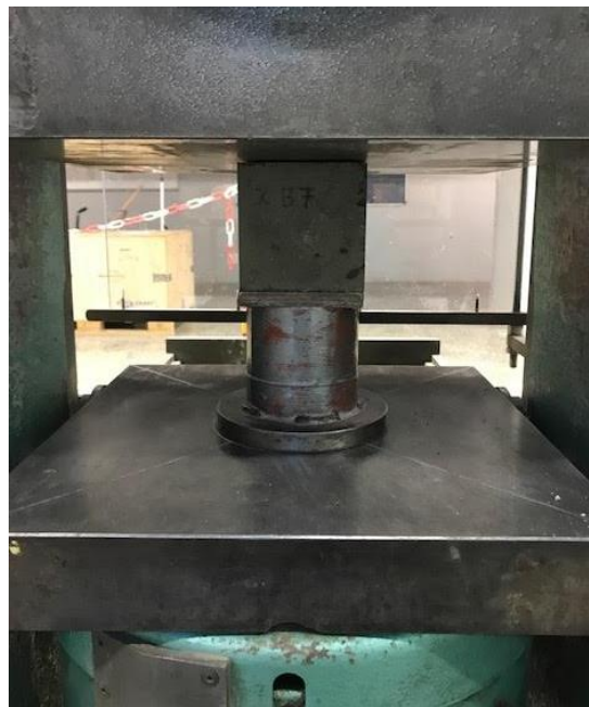
Figure 3.6: Image showing a cube sample centred in the platen of the hydraulic press (Amsler compression tester)
