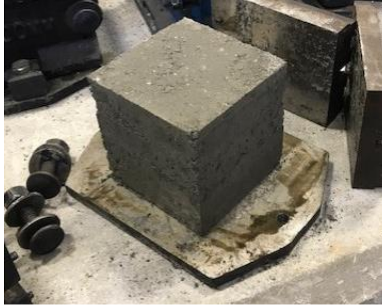
Figure 4.3: Image showing de-moulded sample for the green state strength test.
