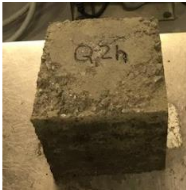
Figure 4.4: Image showing sample Q2H, which has two visibly uneven corners and 10 g of lost material.
