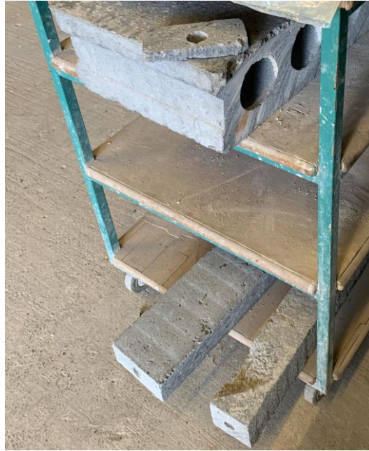
Figure 3.1: Image showing A. 155 x 595 mm hollow core sample, B. 145 x 65 mm lintel and C. 80 x 88 mm lintel.
