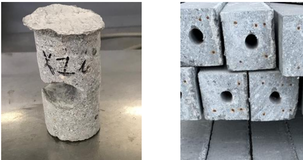
Figure 3.2: Images showing a typical core sample with a void from extrusion, an uneven top surface (left), and the lintel profile in the cross-section from which it was cut (right).
