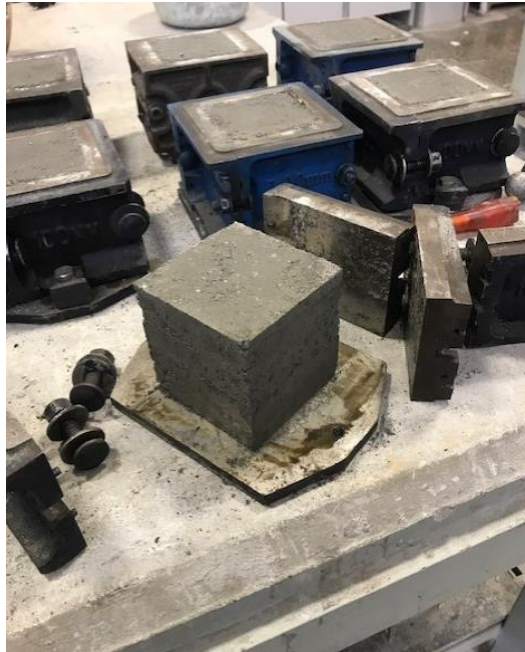
Figure 3.5: De-moulded sample for the green state strength test
