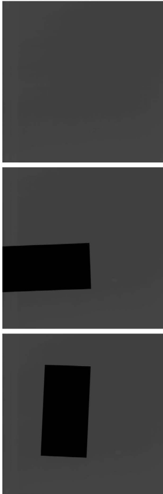
Figure G.1: Sample NPS and MTF Images. Top – NPS, middle –transverse MTF, bottom – lateral MTF.
