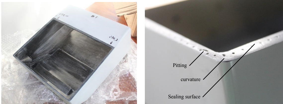
Figure 5.8: CFRP Housing #1. Left – the CFRP housing is shown as delivered. Right – some of the manufacturing issues are highlighted.
