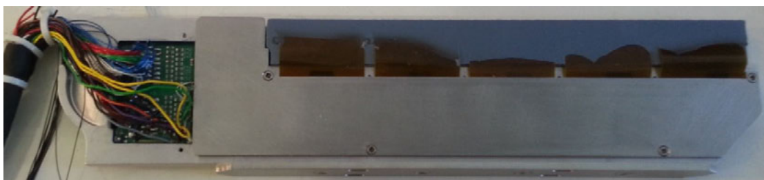
Figure 5.6: Assembled Ultrasound Chassis
