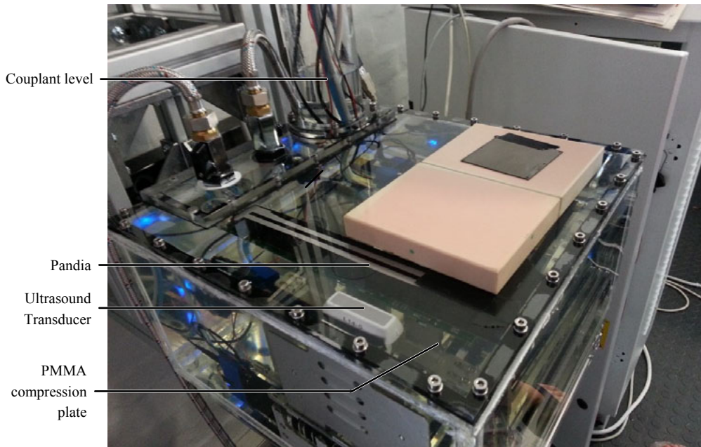
Figure 3.8: Prototype 2 in Operation. The Pandia and ultrasound transducer are shown scanning radiographic tissue clocks from within the PMMA box which is filled with non-conductive mineral oil.
