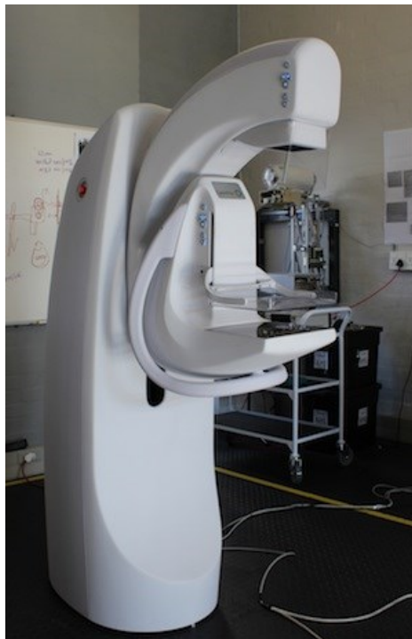
Figure 1.2: CapeRay Soteria. A prototype version of the Soteria; the X-ray only variation of the PantoScanner.
