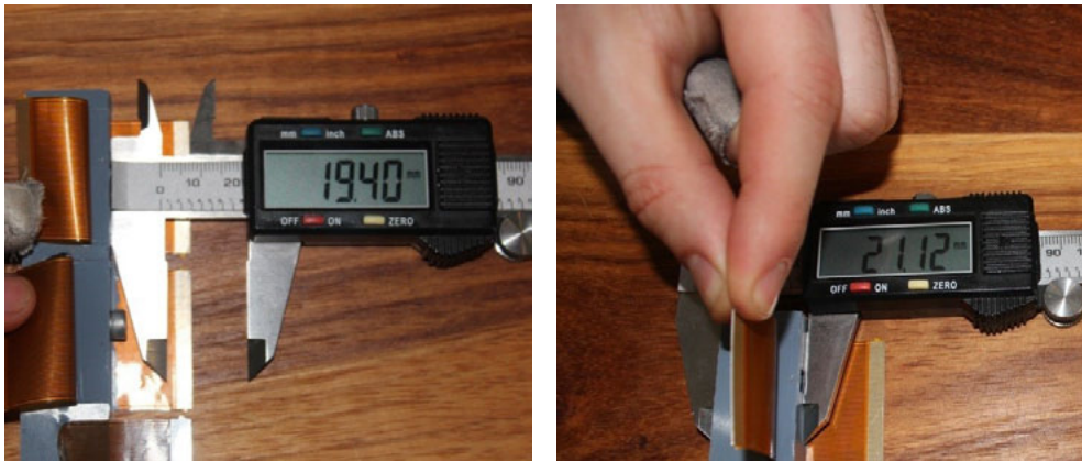
Figure 5.4: Ultrasound Transducer Manufacturing Errors Left – the FPCs are 3 mm shorter than specified. Right – the height of the probe is ~1.5 mm greater than specified.
