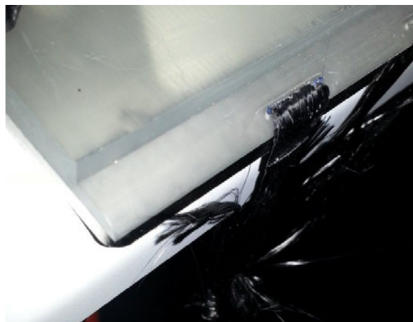
Figure 4.23: CFRP Custom Hook Prototype
