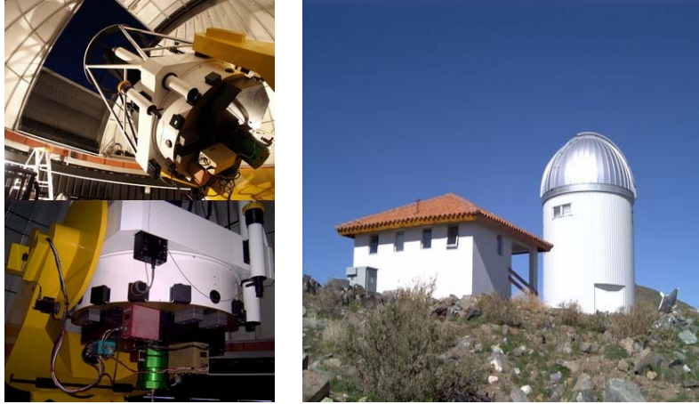
Figure 2.5: Left: The telescope and its CCD camera. Right: Control building and the dome (Adopted from http://ogle.astro.u.edu.pl/main/tel.html ).
