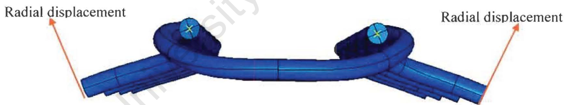
Figure 3-13: Direction of motion permitted for the wire-loop end surfaces at the right and left sides of the assembly (Boundary condition A).
