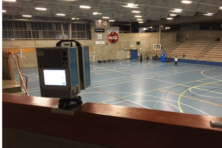
Figure 8.33: Image of the laser scanner running a test scan to analyze the field of view from this location.
