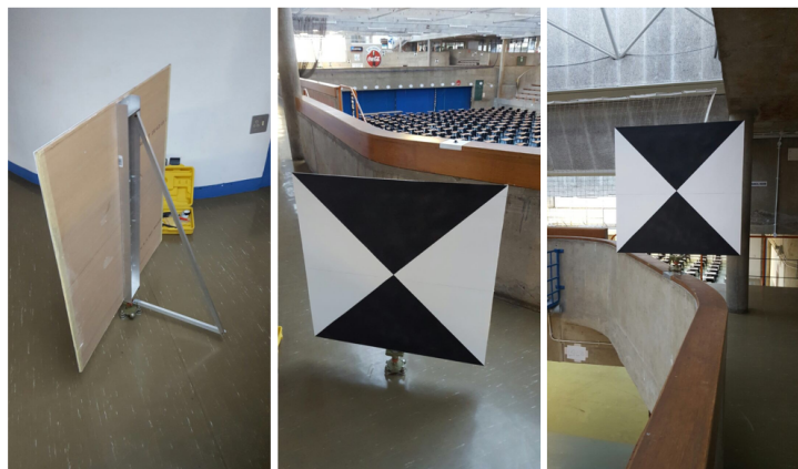
Figure 4.6: Image of the improved target designed for the distance accuracy testing in the medium testing facility, this design was 90cm by 90cm and was the final of two designed for this test.
