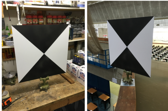
Figure 4.5: Image of the target designed for the distance accuracy testing in the medium testing facility, this design was 50cm by 50cm and was the first of two designed for this test.
