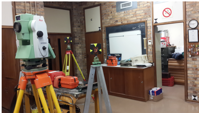
Figure 5.6: Image of the Total Station at work with the prisms and targets in the short range testing facility.
