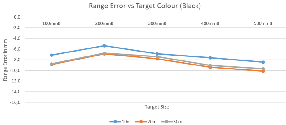
Figure 8.6: Graph showing the same errors in the range between the laser scanner and the surveyed distance but based on on the black targets alone.
