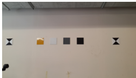
Figure 5.3: Image of the intensity targets positioned in the short range facility.
