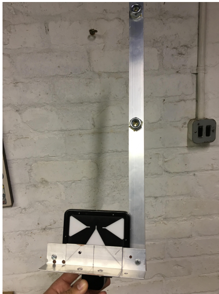
Figure 8.1: Design of the target holder attached to the target that is normally included in a forced centring kit. This target was used because of the ease to attach itself to the rest of the forced centring kit as opposed to fabricating a new attachment.
