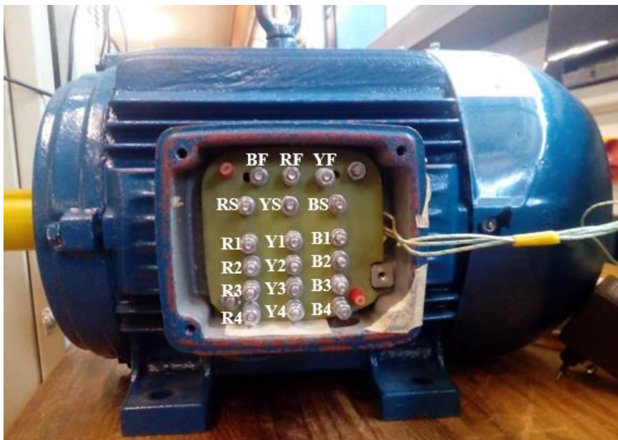
Fig. 6.4: External tapplings of SCIM2 stator winding per phase.
