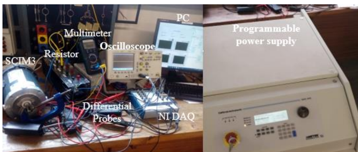
Fig. 6.12: Experimental setup for broken rotor bar fault detection using locked-rotor test
