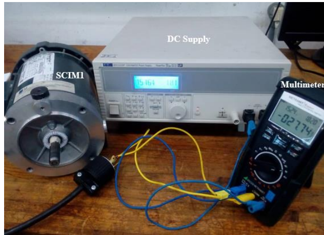
Fig. 6.5: Stator winding DC measurement for SCIM1
