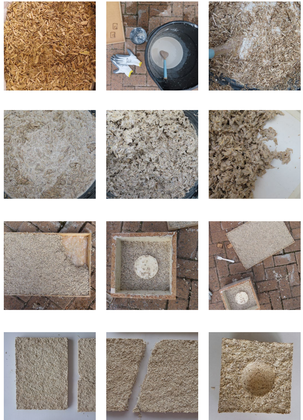
Figure 78 (all images on right): photographic representation of the process followed for making 2' hemp panels and a square brick. Hemp-shiv was combined with a lime binder and water to create a moist mixture that was then tamped into shape and left to dry. The square brick investigated the effect on cast hemp if indentations were made into the wet hemp mixture.
