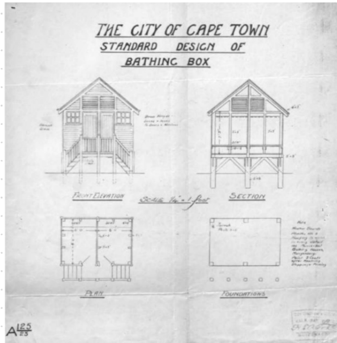
Figure 50: the standardised design for a double bathing box, also designed by Mr Howells in 1910.
