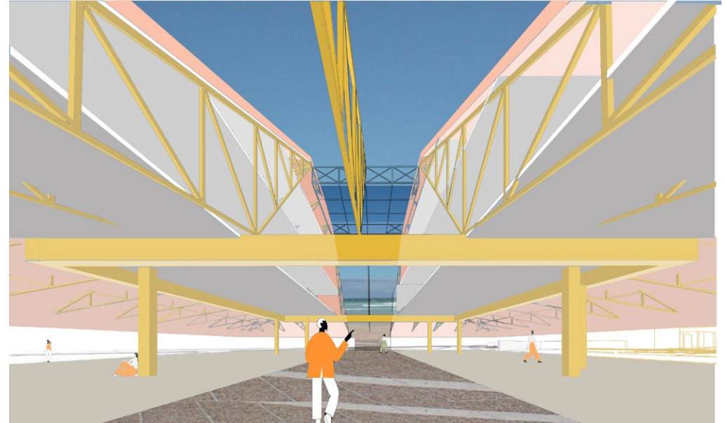
Figure 103: conceptual design presented at the first review illustrating the insertion of 3 additional levels inside the building. The split in the building was an attempt to bring additional light and ventilation into the centre of the building. However, the overall design was dubbed as being too polite and not transformative enough. It was the beginning of a space-making as opposed to the desired form-making exercise.
