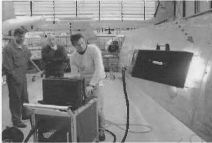
Figure 2.23: Mobile Shearographic equipment applied on an aircraft wing [53]
