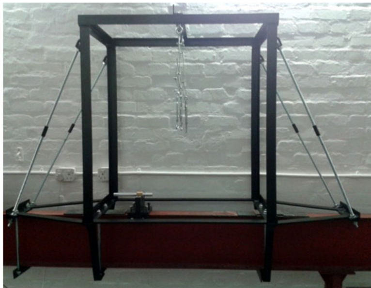
Fig. 5.1 The suspension system utilised in the tests. The specimen hangs upside down in a net suspended by the cables. Turnbuckles allow for easy adjustment of the specimen position.
