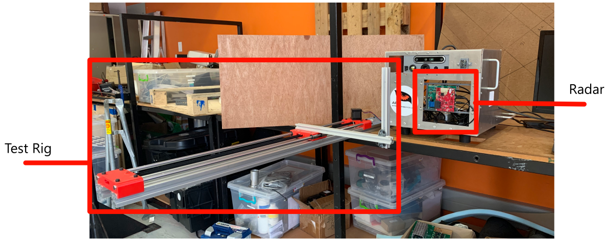
Figure 55: Linear motion rig used to validate the pipeline.
