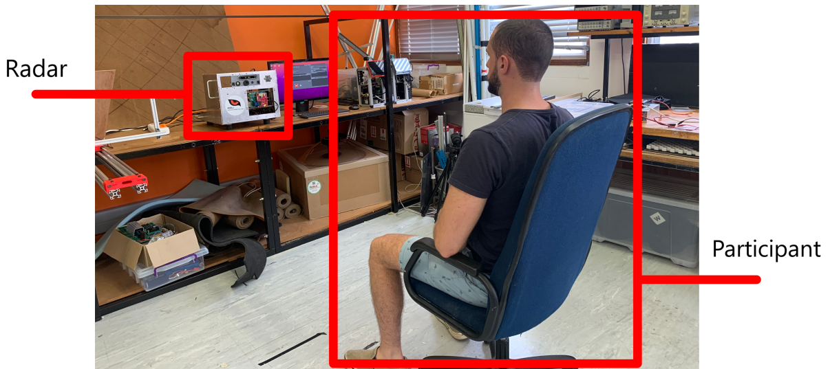
Figure 56: Setup of seated stationary experiments for vital sign measurements.
