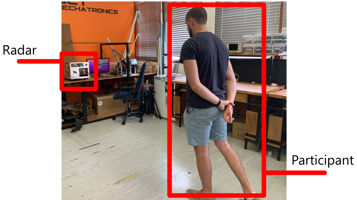
Figure 58: Setup of walking experiments for heart rate and breathing rate measurements.
