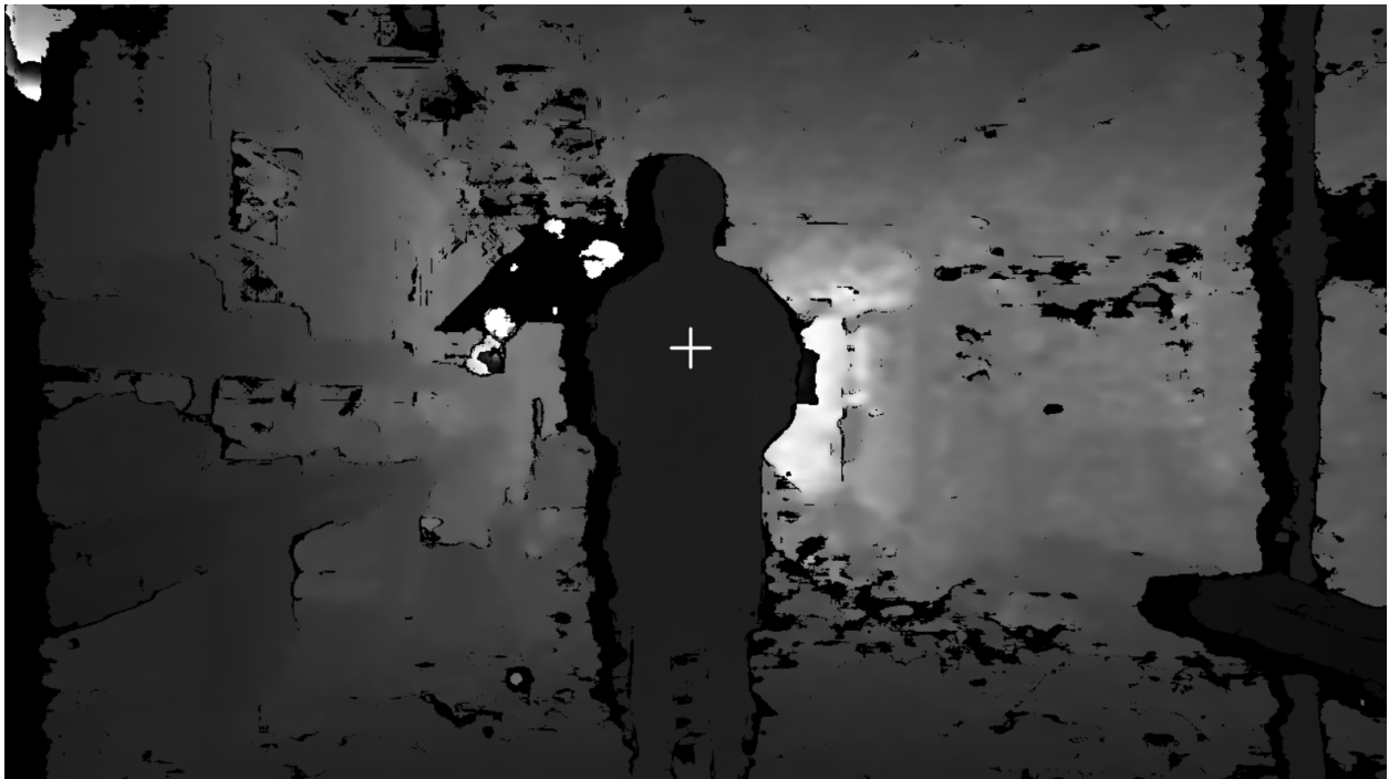
Figure 39: Example output of the RealSense depth data. Image shows the depth of a lab with a person standing in front of the camera.
