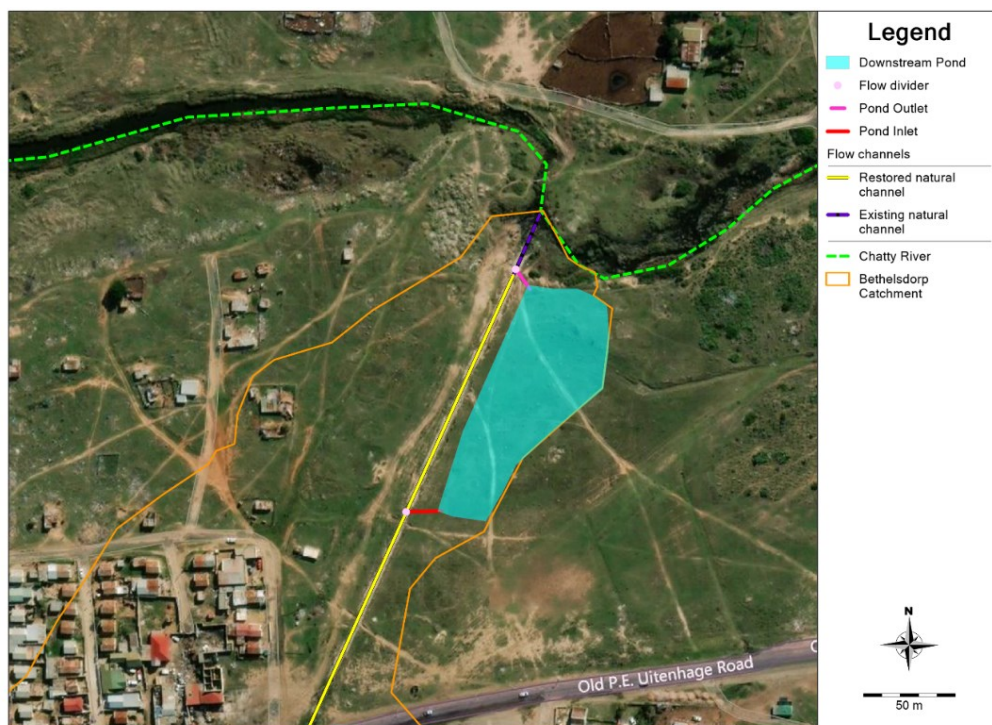
Figure 8-8: Scenario 3: Proposed downstream retention pond
