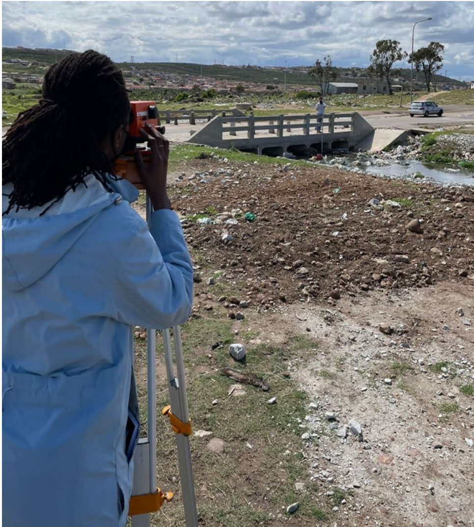
Figure 5-10: Taking slope measurements at Site 5 (Kemps Kloof) using a dumpy level
