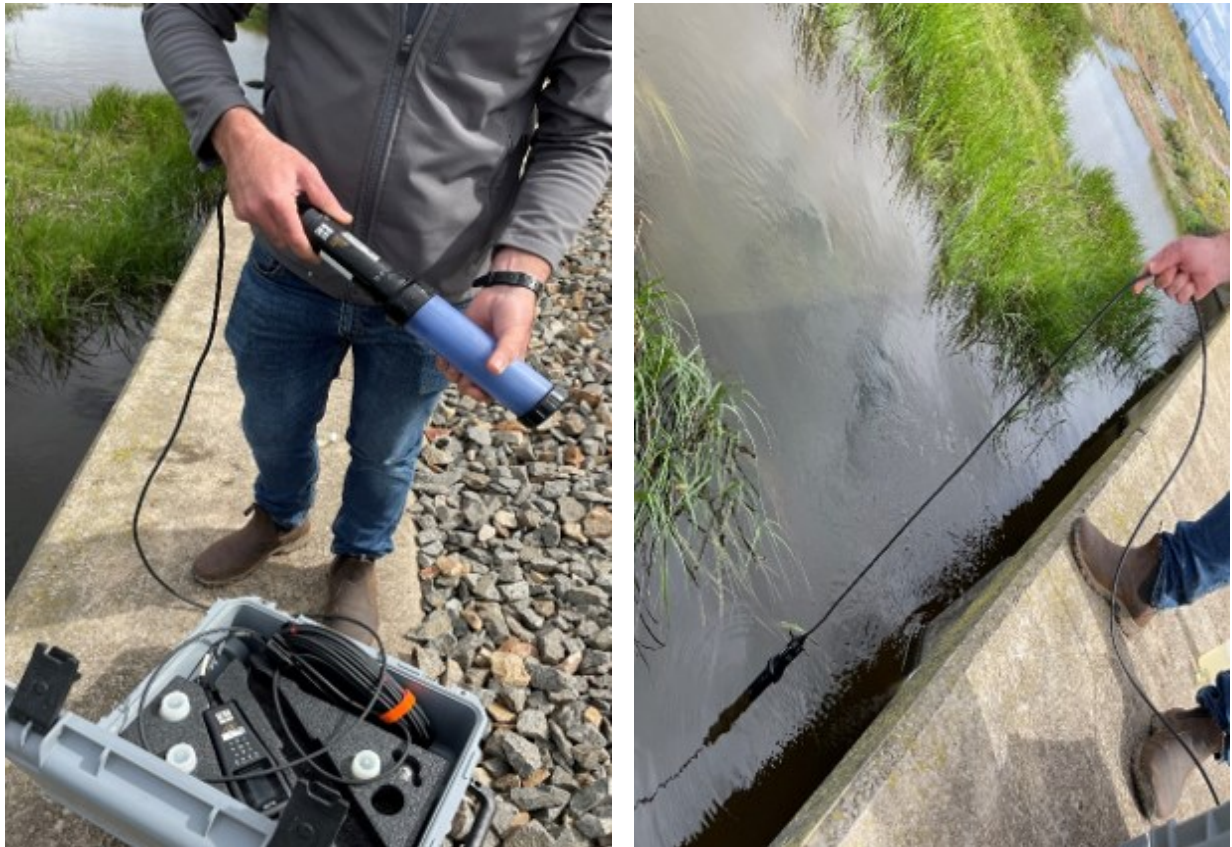
Figure 6-3: Calibration and in situ testing using the YSI ProDSS Multiparameter Digital Water Quality Meter
