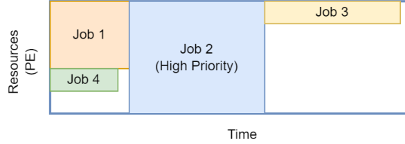
Figure 4.6: An illustration of the backfill calculation process. Three diagrams are shown to breakdown the process, with each diagram showing the job allocation in the dimension of time and PE resources. In the first diagram, four jobs are shown, with some available space currently available which would allow jobs to be backfilled. In the second diagram, the same jobs are shown but with an additional distance measure (referred to as the 'Maximum backfill runtime') is calculated to quantify how long the current available resources would be available for the purposes of backfill scheduling. In the third diagram backfilling occurs according to the implementation in the model.
