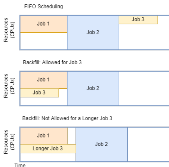
Figure 2.6: An illustration of Backfill scheduling. Three scenarios are shown, each scenario showing the job allocations across time and the CPU resources. The first diagram shows an example of FIFO scheduling where three jobs of different sizes were run in order. The second scenario shown is an example of successful backfill scheduling, where it was possible to execute Job 3 earlier, without delaying any previous jobs. The third example shows an example where backfilling scheduling is not possible, as it would delay the starting time of a previous job.
