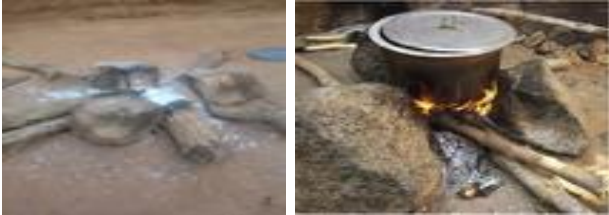
Figure D4.1: Open Fire/ 3stone Stoves
