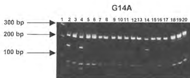
Figure 4.1g: Msp AI restriction analysis of the PCR product of fragment 1 to identify the G14A mutant. Lane 1, bp markers, lanes 2, 4, 14 are wild type clones (post-digestion) and lanes 3, 5-13 and 15-20 positive clones.
