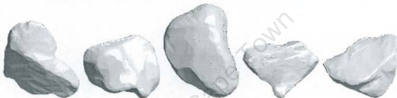
Figure 10.3: Refined visual hull models of stones whose minimum sieve bin is smaller than the minimum cylinder diameter by the largest amount.
