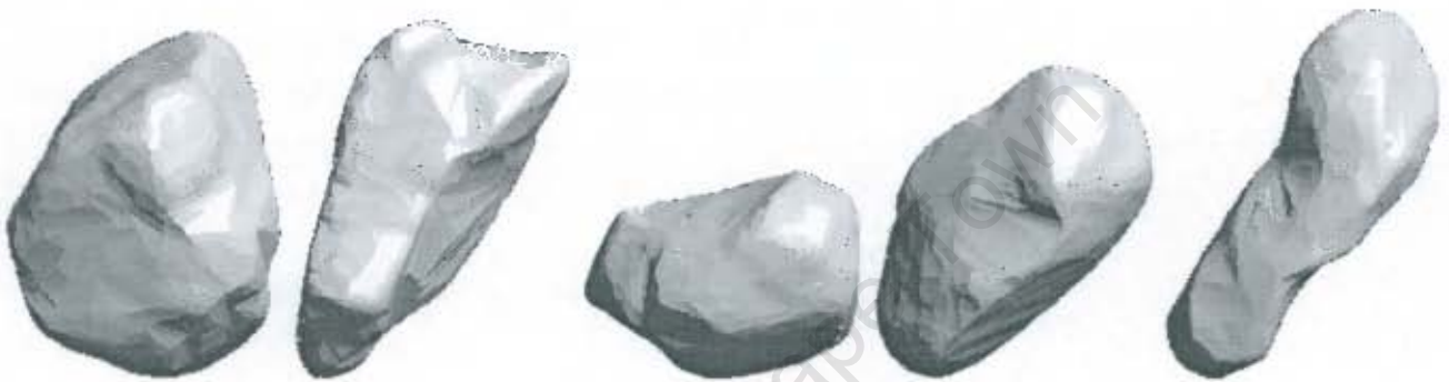
Figure 10.7: Refined visual hull models of stones that tend to fall in different bins as measured by contribution to \Sigma VAR.
