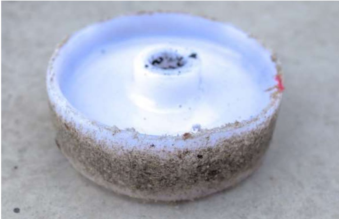
Figure 11 Damaged Wheel Removed from Cart After Bearing Fell Out.
