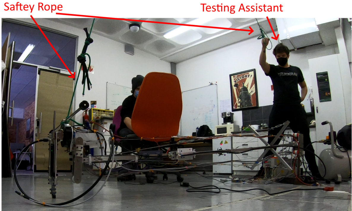
Figure 8.1: Testing procedure with safety rope and testing assistant.
