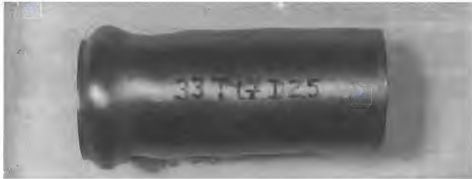
Figure 3.10: Dynamic plastic buckling. The permanent profile of an aluminium cylindrical tube subjected to an axial load. [47]
