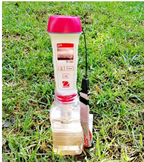
Figure 7-1: Measuring a water sample with the pen meter
