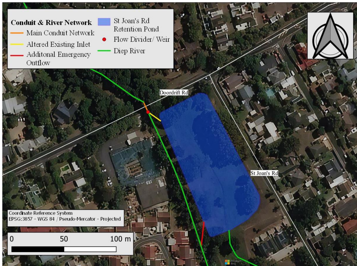
Figure 8-18: Proposed St Joan's Road Retention Pond Layout – adapted from Bing Maps (Microsoft Bing, n.d.)
