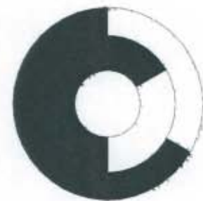
FIGURE 5.9: TWO TRACK ENCODER
