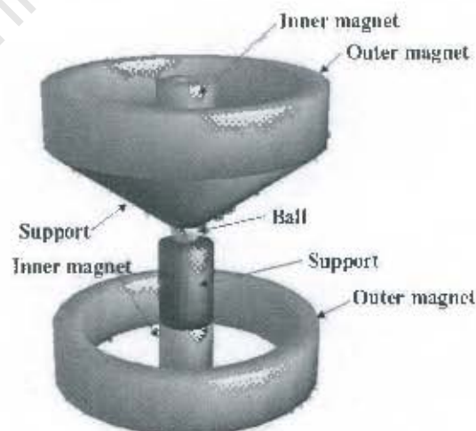
FIGURE 2.12: HYBRID MAGNETIC BEARING CONSTRUCTION
