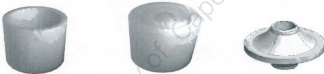
FIGURE 4.1: THIN CYLINDRICAL FLYWHEEL , MULTIPLE RIM FLYWHEEL AND ULTIMATE SHAPE FLYWHEEL.
