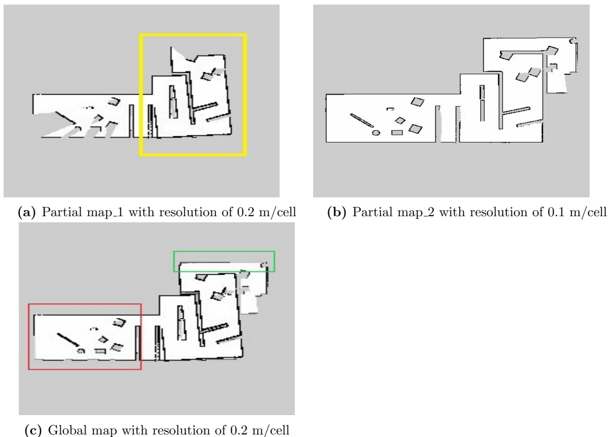
Figure 5.12: Two partial maps and a global map are presented. The partial maps are generated from simulated data, and they are of varying resolution. Since the maps are aligned relative to map_1, the resultant global map will have the same resolution as partial map_1. In (a), the yellow region highlights a mapping error in map_1. In (c), the resultant global map shows the mapping error in map_1 being propagated, highlighted by the red and green regions.
