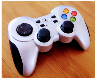
Figure 5.21: The Logitech Wireless Gamepad F710 uses a powerful and reliable cable-free 2.4 GHz connection while dual-motor vibration and is used to control the Kobuki Platform.
