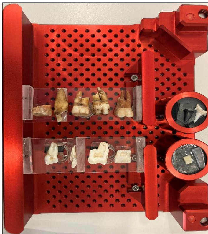
Figure 7: Teeth ready for analysis in the sample chamber of the LA-MC-ICP-MS.
