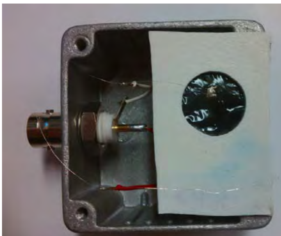
Figure 4.1: Left is a schematic diagram of nanowires array in a template with conductive paste on top. Right is a picture of the box used in our measurements. A hole is drilled for the BNC connector which can be soldered to any template that needs to be measured. The template is supported by the same insulating rubber sheet used in the electrodeposition process.
