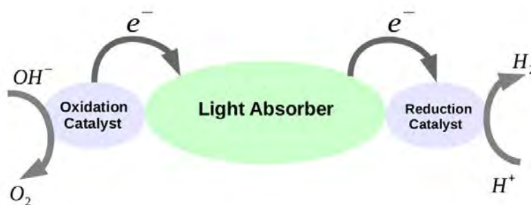
Figure 5.1: Schematic diagram of an effective photocatalyst structure. Three essential components are needed: a light harvesting material (semiconductor), an oxidation electrocatalyst, and a reduction electrocatalyst which facilitate the desired chemical reactions.
