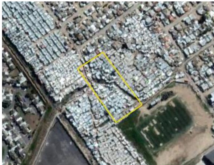
Figure 38: An example of a pond invaded by an informal settlement
