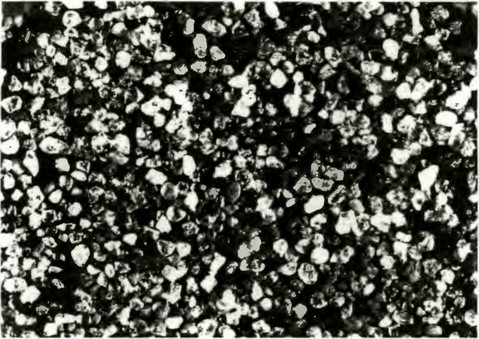
Plate 13: ELS 3 - fine-grained quartz sand, with numerous fragments of weathered Malmesbury shale/laterite/ferricrete (linear magnification = X20)
