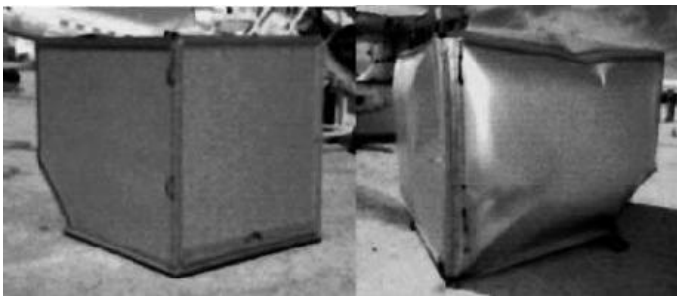
Figure 2.5.1: Cargo hold prototypes made from GLARE, shown before and after blast loading [3].
