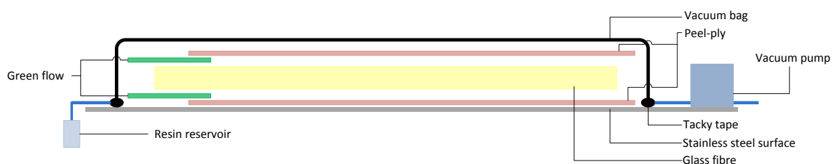
Figure 3.3.2: Vacuum Assisted Resin Transfer Moulding configuration of GFRP laminate
