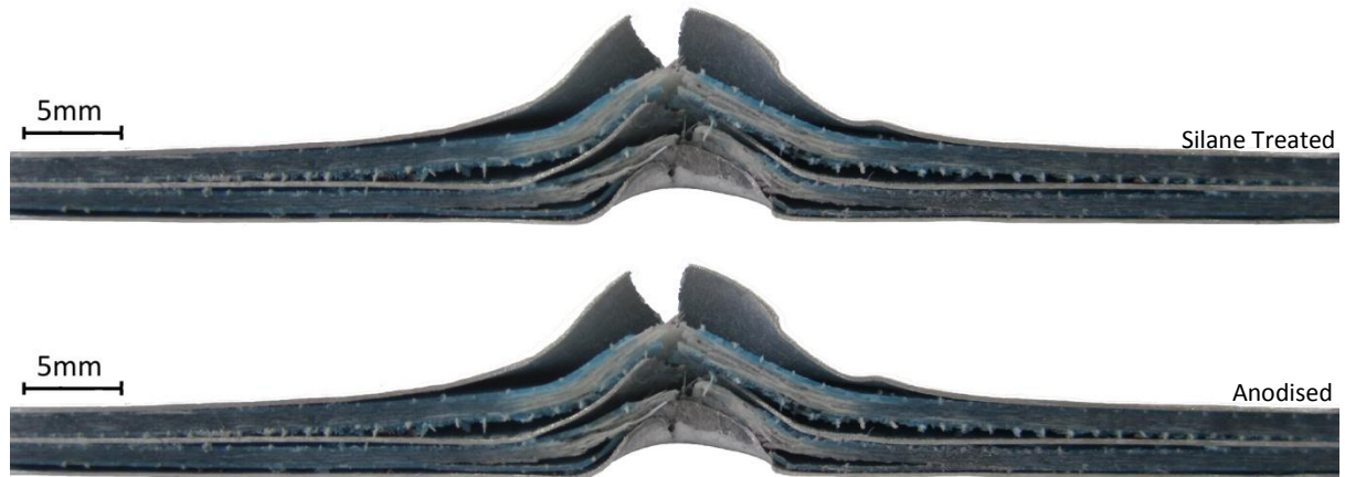
Figure 5.2.4: Photographs of FML cross-sections, ISS 8 (top) and ISA 3 (bottom), subjected to the same non-dimensional energy (0.034)
