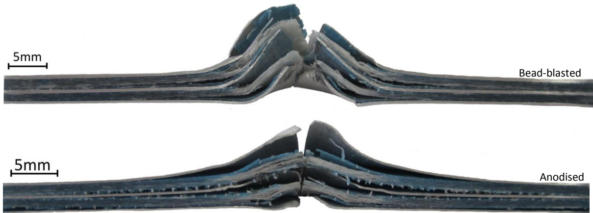
Figure 5.2.6: Photographs of FML cross-sections, ISG 2 (top) and ISA 10 (bottom), subjected to the same non-dimensional energy (0.041)
