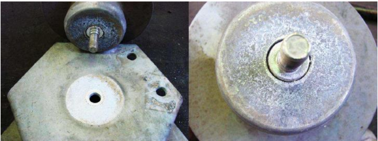
Figure D. 13 Faulted Umfolozi – Bloedrivier Areva surge arrester sent to RT&D unit before dissection [78]
