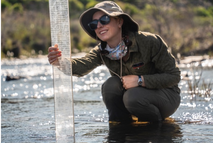
Figure 2.4. Photograph of the use of the transparent velocity-head rod (TVHR) used for the collection of velocity measurements during the 2021 sandfish microhabitat use surveys in the Biedouw River. It is placed into the water column with the broad face turned into the direction of the flow. Two measurements are then taken: the superelevated depth on the upstream face and the depressed depth on the downstream face. Photograph by Jeremy Shelton.
