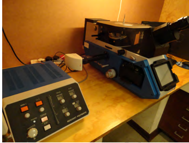
Figure 3.9: Reichart MeF3A inverted light microscope fitted with a polarized lens.
