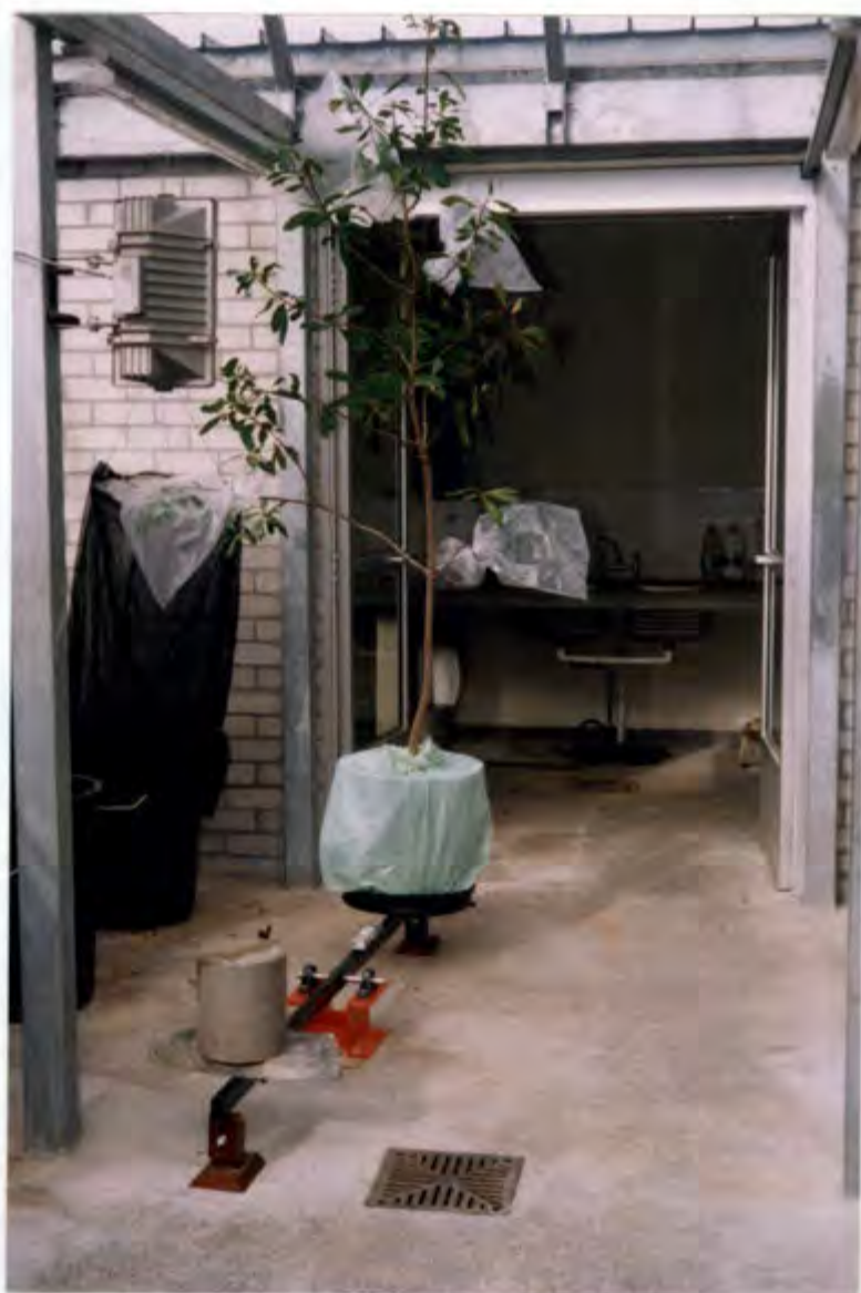
Figure 1. Experimental set-up for testing the accuracy of the deuterium tracer method on Rapanea melanophloeos using a gravimetric technique.
