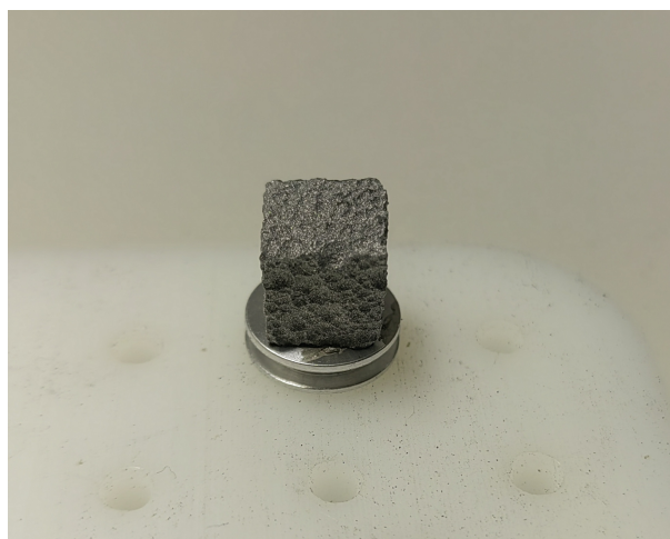
Figure 3.9: AA8021-AC solid sample on SEM specimen stub after deep etching (partial dissolution)
