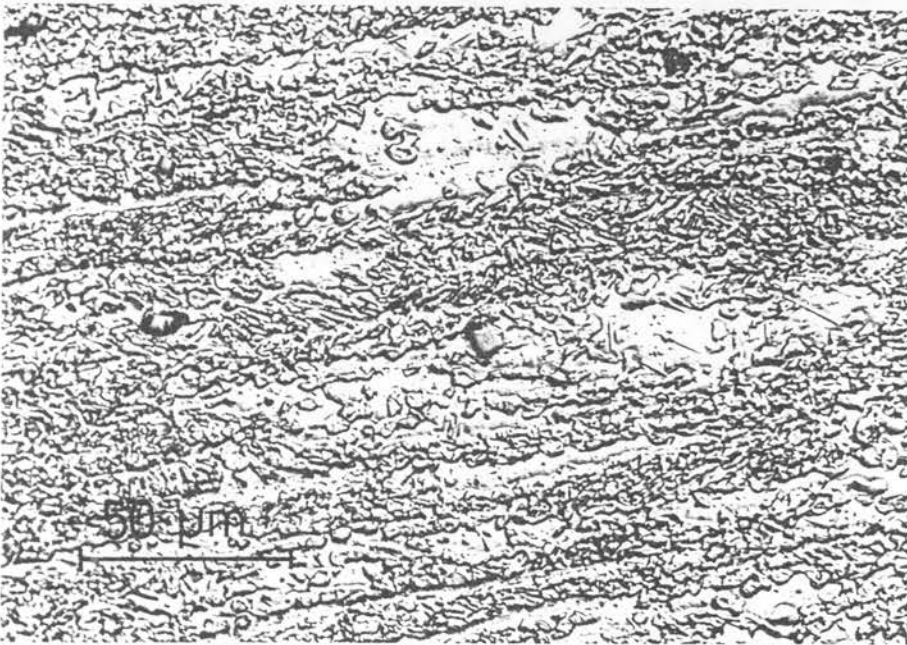
Photo 5.11 As-received + quench from 778°C HV 30 : 231
