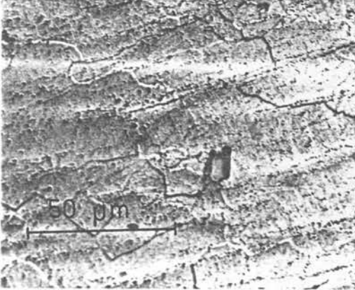
Photo 5.6 Quench from 778°C HV 30 : 141 VPM: 0%
