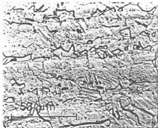
Photo 5.9 Quench from 952°C HV 30 : 270 VPM: 91%
