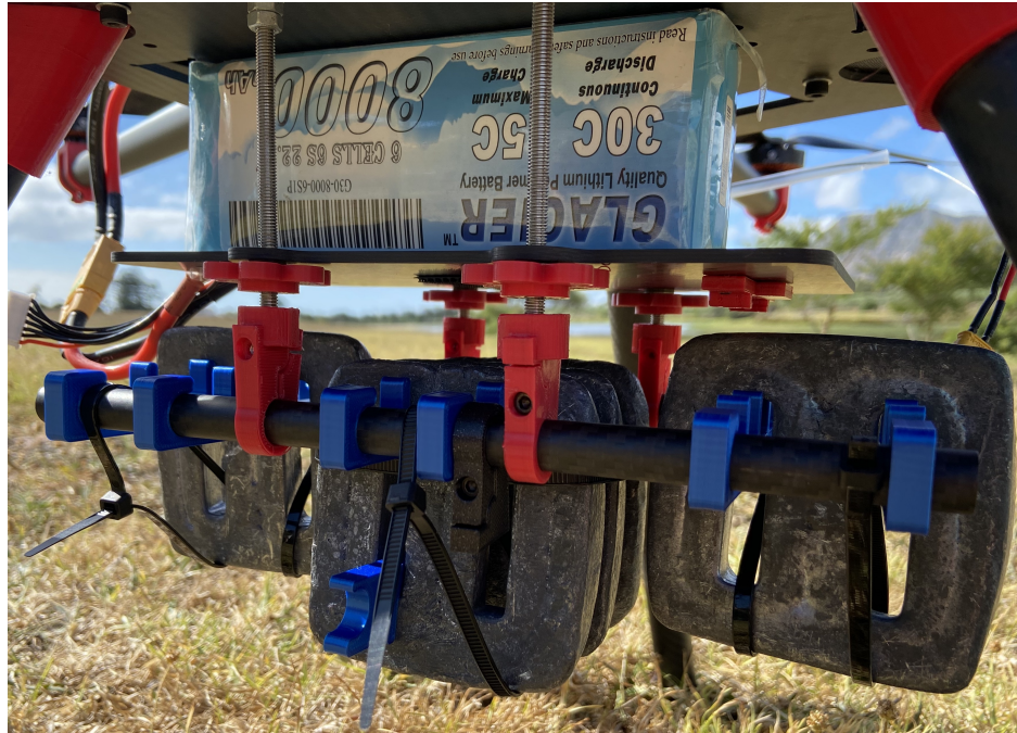
Figure 6.9: Illustration of how the weights were mounted onto the HexaQuad gimbal rails for payload testing. A 3D print snap on mount supported the weights while zip ties were used to prevent the weights from shifting during the tests.
