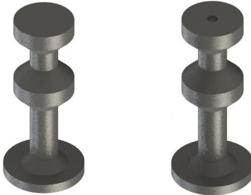
(a) CAD model showing the press with the flat face used to compress the PE4 into place.
