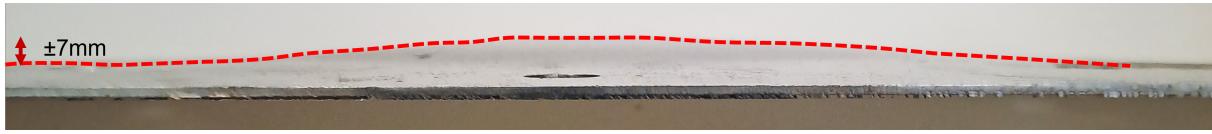
(a) Typical deflection observed from a complete target plate.
