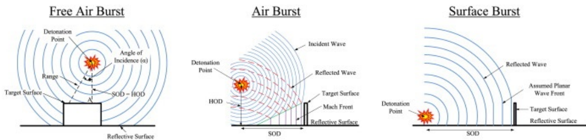
Figure 2.8 Illustration depicting the varying levels of unconfined blasts. [44].
