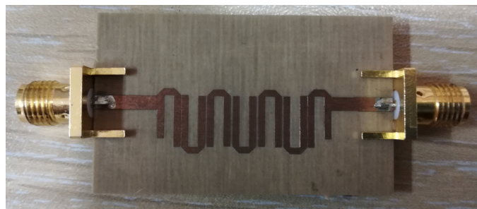
Fig. 5.14. Image of the microstrip hairpin filter.
