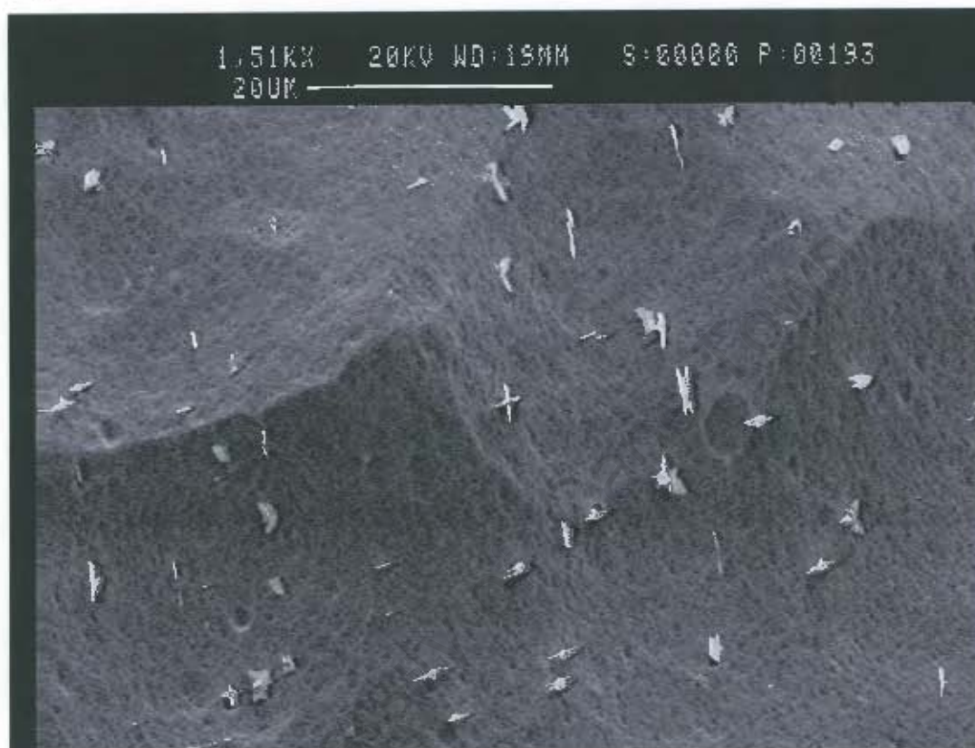
Figure 4.3: SEM micrograph exhibiting the general morphology of the precipitates found in the tundish sample (1500X)
