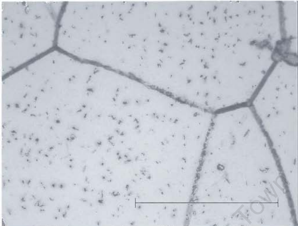
Figure 5.10: Micrograph of the material 3 of the material after sag testing. 1000X magnification micron marker = 50 \mu m.
