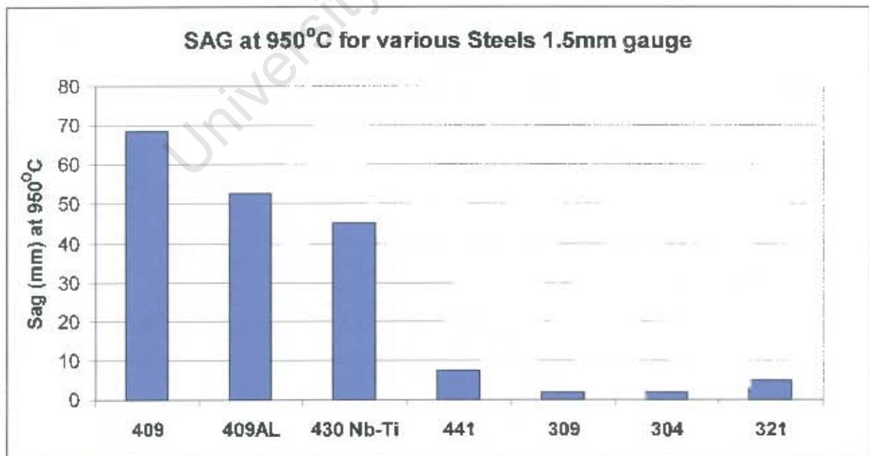
Figure 3.4: Sag resistance of various steels tested at 950°C for 100hrs (1.5mm gauge) (63)
