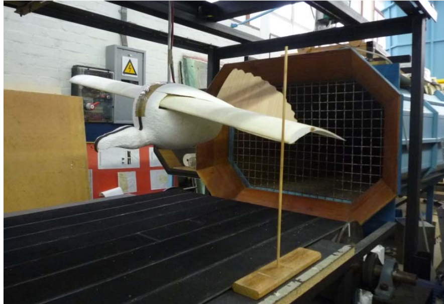
Figure 3.29: Figure showing Vertical Placement of Model in Wind Tunnel with back Region of Tail at Boundary of Airflow
