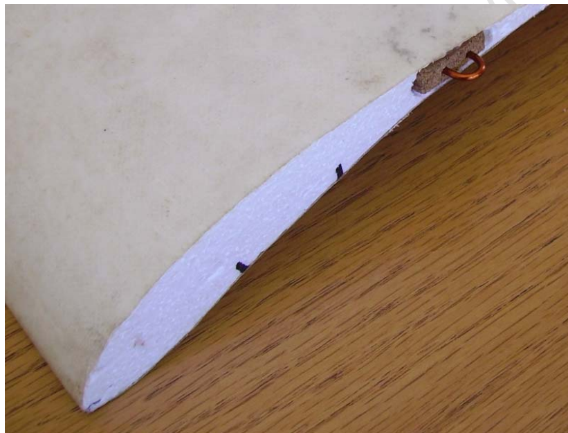
Figure 3.7: Figure showing the Measurement Point for the Experiments involving the Roll and Yaw Axes
