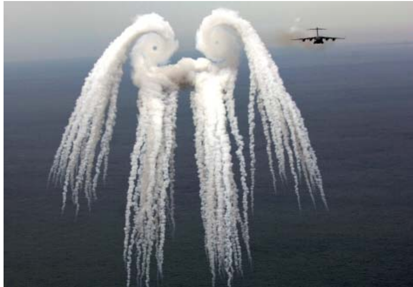
Figure 2.7: An impressive Demonstration of the Effect of Wingtip Vortices [8]. The spiral-like shapes that this smoke bomb has been drawn into are the result of pressure gradients generated around the wingtip.
