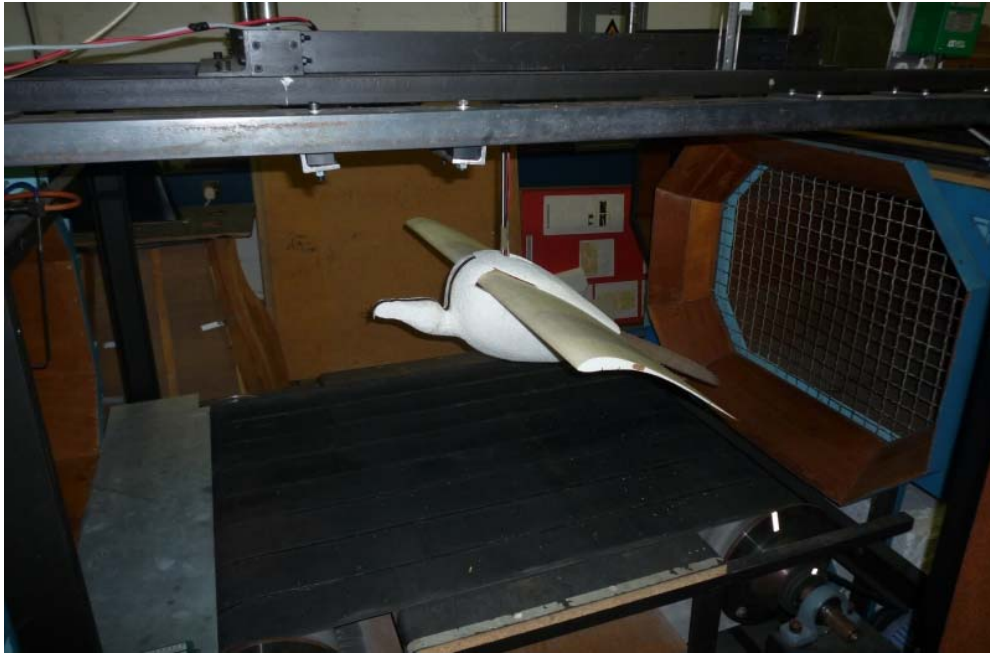
Figure 3.24: Model mounted in Wind Tunnel without Airflow
