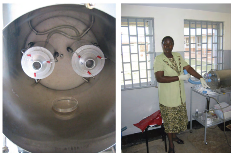
Figure 36. Cough aerosol sampling system (CASS). View inside the sampling system with two Six-stage Viable Anderson Cascade Impactors (VACIs) and a collection plate (left) and the outside view of the CASS set up in the procedure room (right). Adapted from Fennelly et al., 2012.
