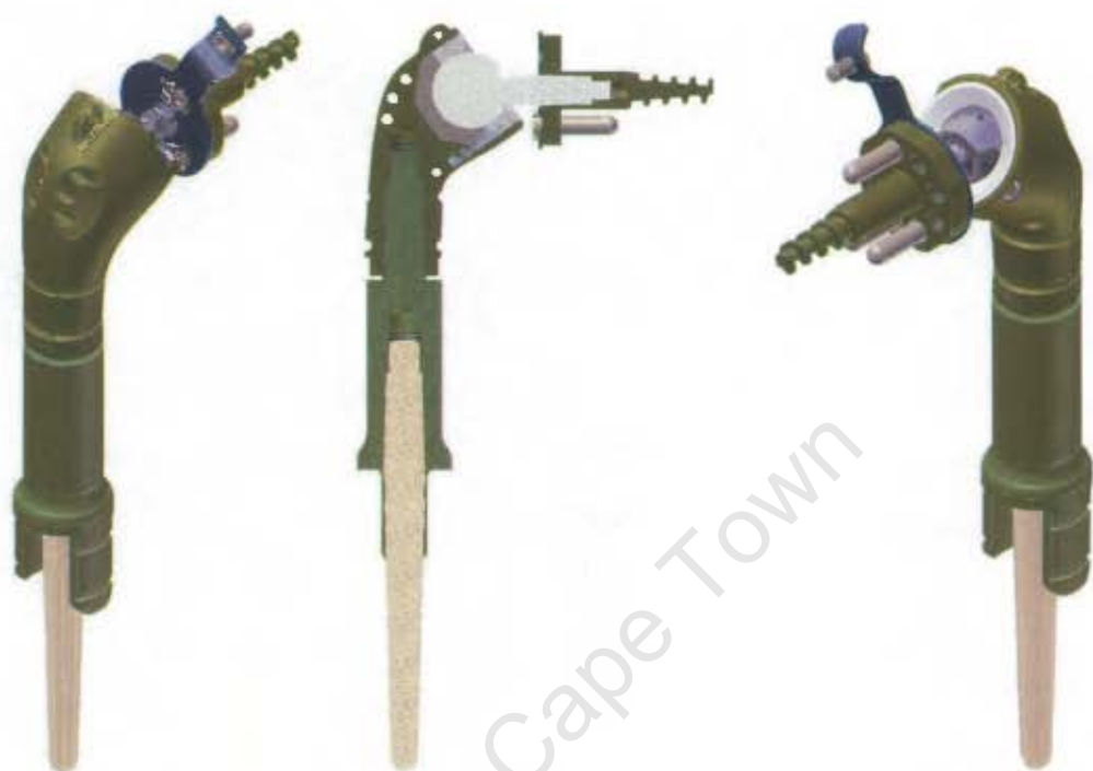
Figure 4.7: The Hybrid-Screw TSR assembly.
