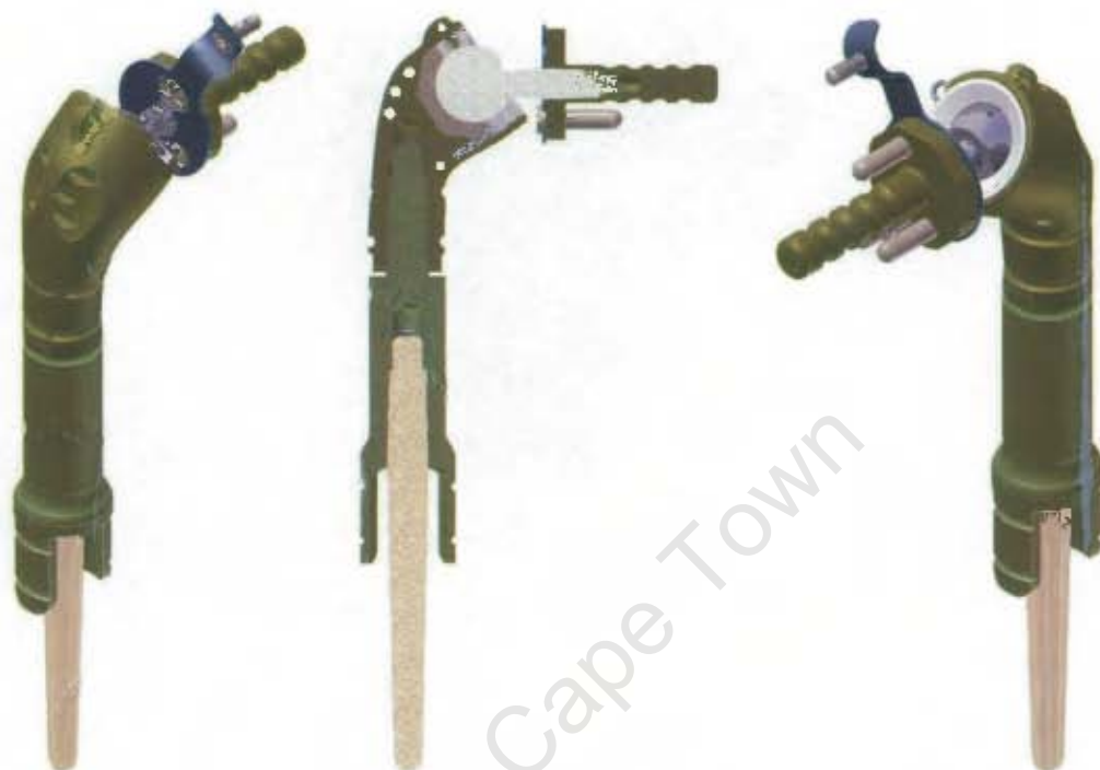
Figure 4.10: The Central-Peg TSR assembly.
