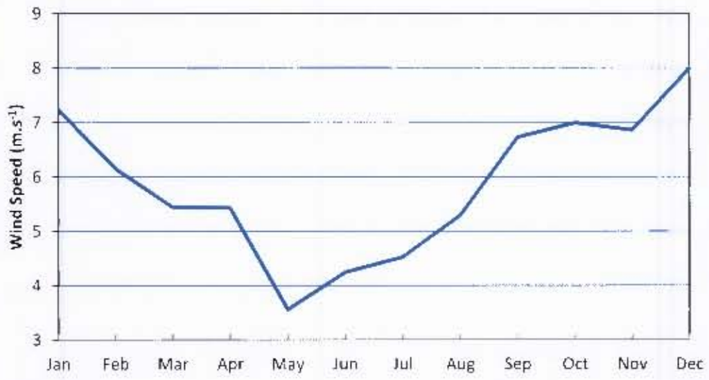
Figure 2.13 Average monthly wind speeds (2008-2009) from anemometer data at the Dias Point weather station, Luderitz.
