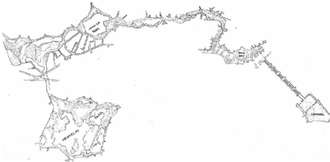
Boston's Emerald Necklace hybrid landscape integrates transportation, flood and drainage engineering into landscapes with recreational and amenity value (adapted from Jellicoe, G. and S. Jellicoe. 1987. The Landscape of Man. , p281)
